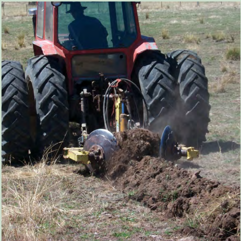
Figure 30: A ripper-moulder being used to create a mounded planting site in a salinity planting. Photo: HLN
