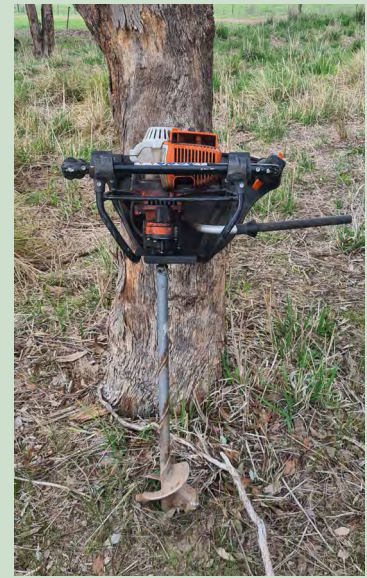
Figure 34: Petrol motor hand augers are an option where ripping is not an option. Photo: Kylie Durant
