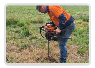
The hand held petrol motor auger is modified so that it does not leave smooth or compacted sides.
