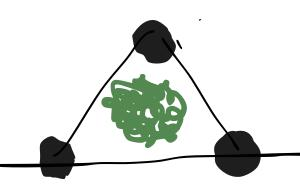
Tree is planted in a triangle of star pickets running three electric wires. The trees are planted about 30 m apart
